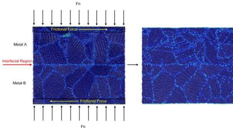
Schematic representation of simulation set-up: Average grain size of 15nm
