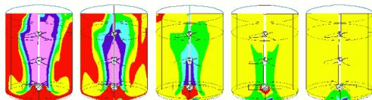
*Normalised tracer concentration versus time, introduced from the inlet for both original and modified design, on a longitudinal plane between two baffles*
