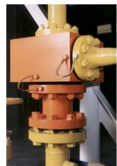
BHR's compact separator, separates the gas from the liquid of the HP flow. The separated liquid is fed into the nozzle of the jet pump as the motive flow. The total LP flow enters the suction line of the jet pump and combines with the HP flow, passing through the mixing tube and diffuser where transfer of energy takes place. The separated HP gas is combined with the fluid mixture from the outlet of the jet pump using a commingling spool.
